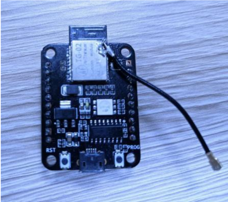
Figure 7 A schematic diagram of the user welding the module to the motherboard
